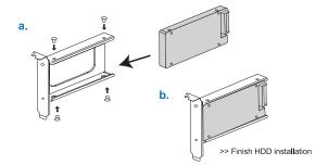
• Mount the bracket to the computer case and secure it with the screw from the PC.
