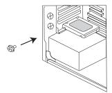
• After the hardware install, connect your SATA and Power cable (not included) to the HDD and power supply. Then you can start using it.
